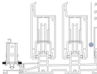
Ample space between panel and riser means panels won't bind
