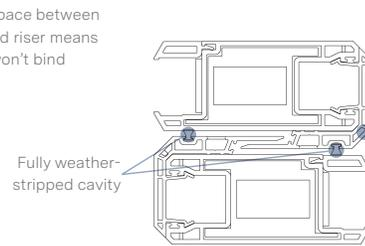
Fully weather-stripped cavity
